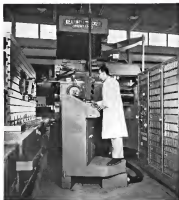
TAPE-PROGRAMMED cutting machine will be used by Martin Co. in P6M SeaMaster and Minitar missile production. Machine was developed by Bechtel Arctech Corp., will provide fast production application of the parasite.
